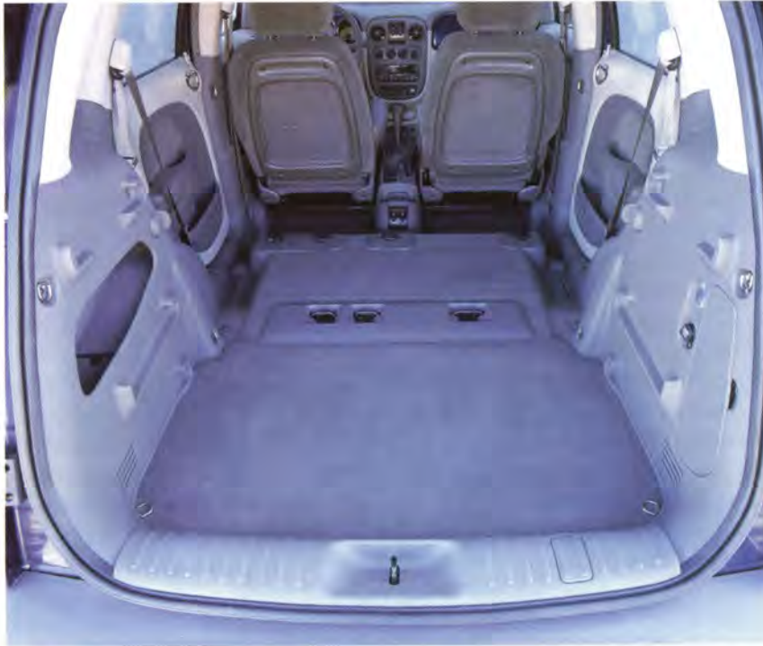
Of the PT Cruiser's interior, one focus group respondent said, “Give me room to the walls and don't tell me how to use it.” As a result, the inside of the vehicle can be configured many different ways, thanks to removable seats and other customizable features. The research showed that the interior had to match the exterior's “wow” factor, otherwise the car might be viewed as a nice-looking package with nothing inside.
